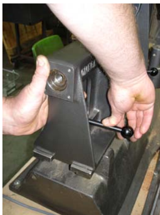
(5) For final adjustment – Place tailstock on bed and tilt top toward headstock. Hold in this position, move locking lever toward you then lift clear of splines, move toward headstock & drop to engage splines and move lever toward you again. Repeat until satisfactory lock up is achieved. NOTE – Locking lever operates in similar way to toolrest lock levers.
