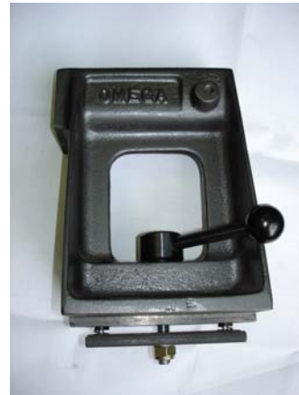
(4) Correct Assembly - Nylox Nut locked up with approx 3/16" thread showing and 5/8 gap between plate and tailstock base.
